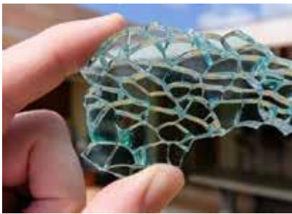
Broken toughened safety glass
