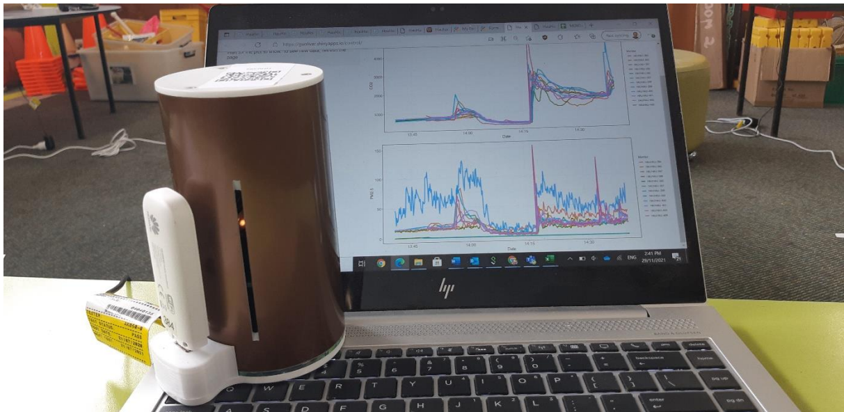
Figure 2-1: A Hau-Hau monitor, alongside a dashboard showing data from ten monitors in the Control Study room.
