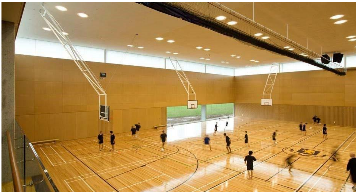
Figure 26: Auckland Grammar School gym sports centre. High level translucent glazing with sloped ceiling to minimise glare. Limited low level windows for view; glare risk mitigated by non-reflective external surface.
