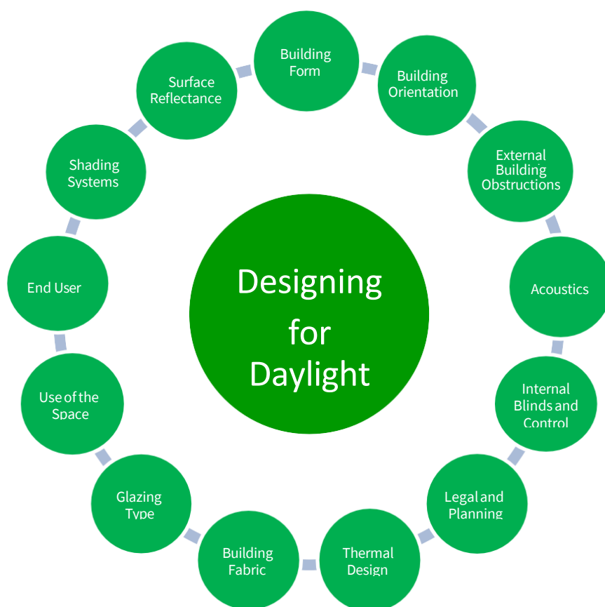
Figure 3: Factors to consider when designing for daylight
